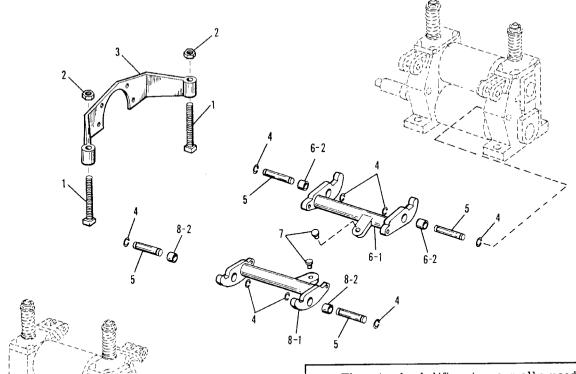
The standard lifter is normally used forblanking progressive and cut-off die work on Open Back Inclinable Presses. It should not be used for drawing or deep drawing work. It is impossible to keep the rolls open for the time required in drawing or deep drawing work without separating them an excessive amount. Normally, the rolls should not be opened more than 1/16" or another roll is not more than twice the thickness of the stock being fed.
